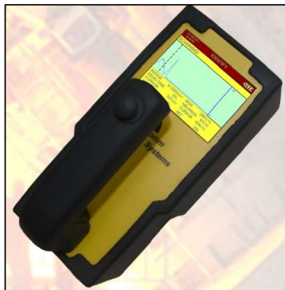
Fig. 11, example of a handheld portable Gamma Ray spectrometer
