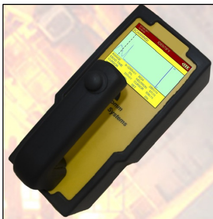
Fig. 11, example of a handheld portable Gamma Ray spectrometer
