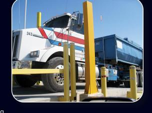
accurate scanning while maintaining a low false alarm rate. If radiation signatures are present in a load of waste or scrap material, the system will immediately alarm and flash red to alert the user that a potential radioactive source has been detected.
