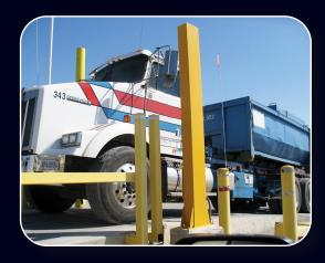
accurate scanning while maintaining a low false alarm rate. If radiation signatures are present in a load of waste or scrap material, the system will immediately alarm and flash red to alert the user that a potential radioactive source has been detected.
