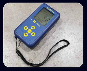
to monitor accumulated dose. Measure not only personal absorbed dose, but locate the unit near the air intake of a building for the tracking of accumulated dose of air filters or intake pathways. Tracking of an air intake filter will provide vital information in determining when to shut down a system or when to change the filter.
